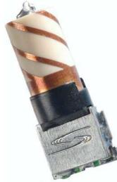
Figure 4 – Sarantel helix antenna (cover removed)
