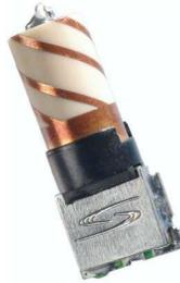
Figure 6 – Sarantel helix antenna (cover removed)
